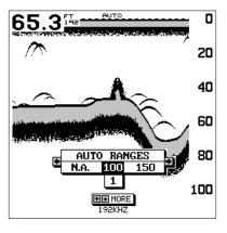
change the range to 150 feet. To do this, simply press the right arrow key while the Auto Range menu is displayed. When you're finished with this menu, press the EXIT key to erase it.
